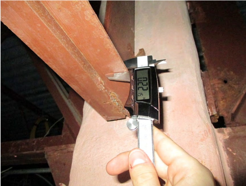
S59 - Caliper thickness measurement of joist bottom chord angle
