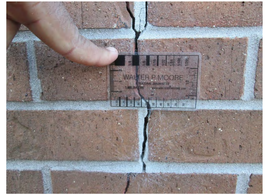
Brick crack width measured as 1/4- inch
