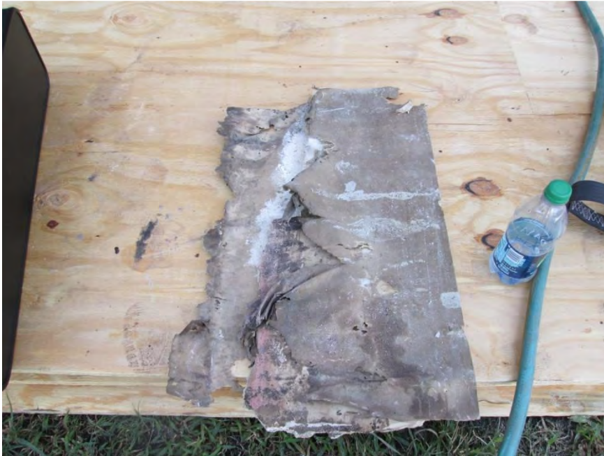
S47 - Moisture deterioration and caking of gypsum sheathing
