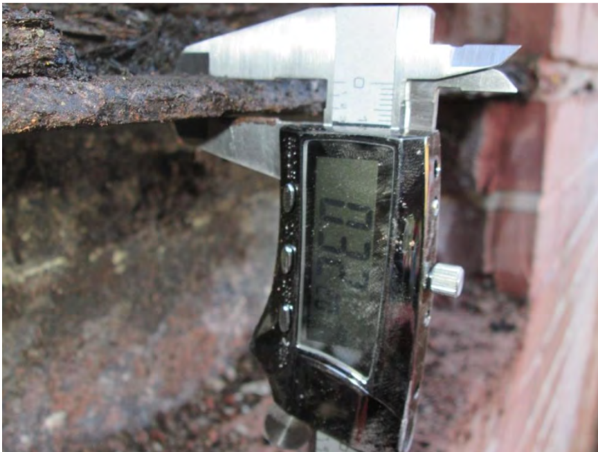
S22 - Caliper measurement of cleaned bare shelf angle leg (~0.32-inch)
