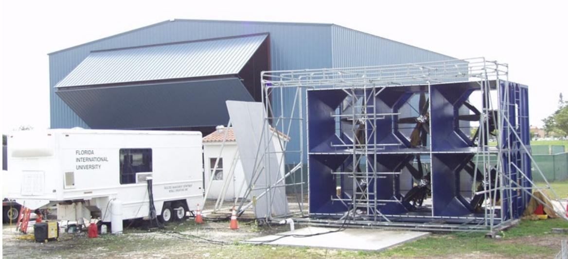
**Figure 1. RenaissanceRe 6-fan Wall of Wind and new 8,000 sq ft facility, which will house the testing apparatus, control room and state-of-the-art, industry-partnered AIR Worldwide turntable.**
